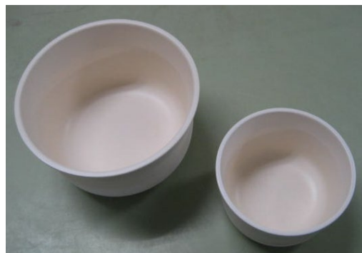
Fig. 3 Photograph of glaze samples with no cracks.
